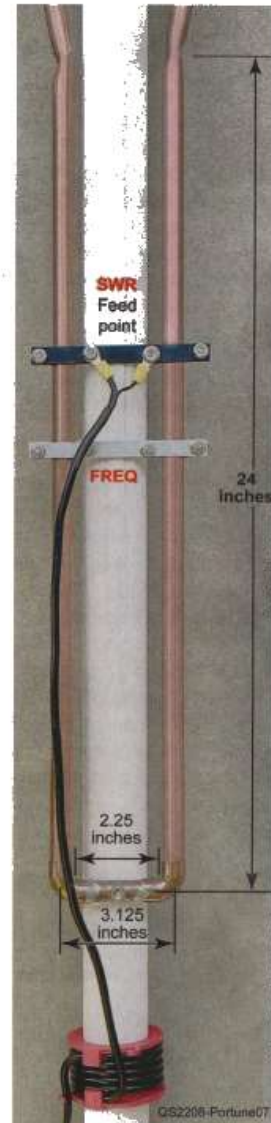
Figure 7 — The adjustment area location and details.
