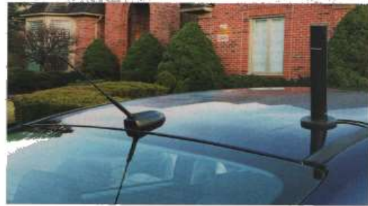
Figure 9 — The COMPACTenna 2M/440+ vehicle installation with the Larsen NMO magnetic mount.
