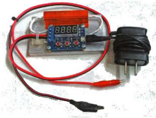
Figure 2 — The mechanical mounting of the load resistor and module. The standoffs provided used metric screws and were threaded. We used sheet metal self-tapping screws, because the heatsink was soft aluminum.
