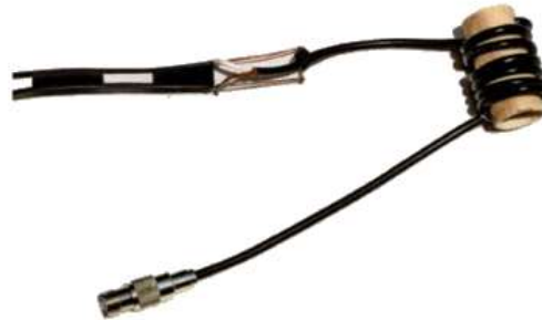
Figure 2 — The J-pole feeding end is on the lower left, and the choke is on the right. [Fred Delaney, K1DU, photo]
