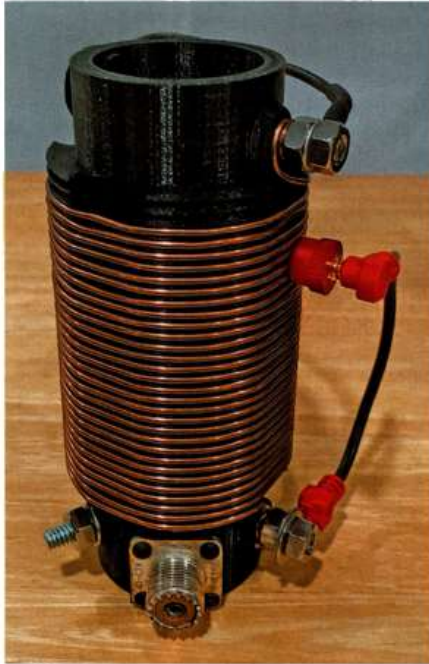
An antenna loading coil for portable use printed with polylactic acid (PLA).
