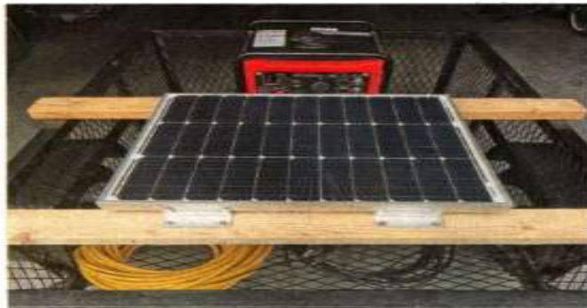
Figure 2 — My small utility trailer with a mounted solar panel and secured Honda generator.
