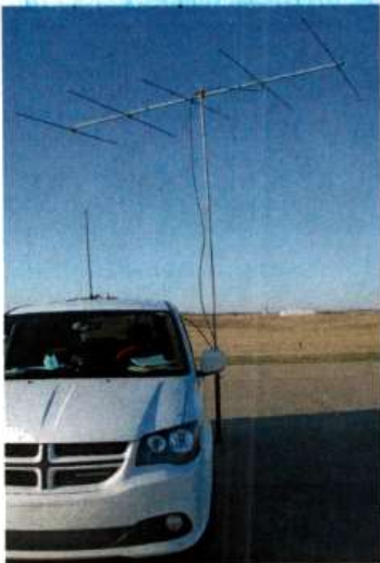
Figure 2 — Larry Lambert's, N0LL, portable 6-meter MSK144 operation. Setups like Larry's can provide amateur radio communications in a natural disaster. [Larry Lambert, N0LL, photo]
